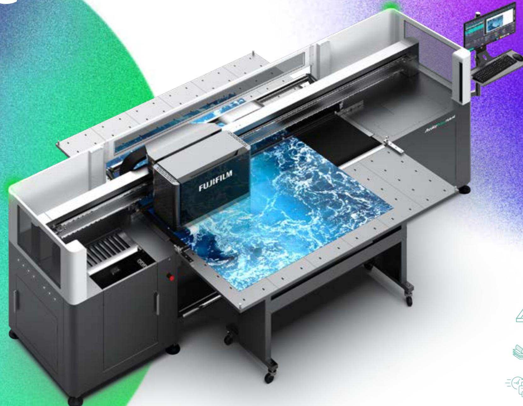
The Acuity Prime Hybrid can be configured with up to 7 channels, with CMYK as standard, and optional White, Clear and Primer, and produces stunning quality print, able to produce droplet sizes down to 7 pL. It handles flexible and rigid media up to 51 mm thick, and roll media up to 2.1 m wide, and benefits from an ultra-reliable and long lasting air cooled LED UV curing system.
